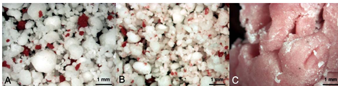
Fig. 3. Dextrin pellets (38.3%, w/w, water) in the equilibrium phase, plain pellets mixed with tracer pellets for different periods ( t_{\text{mix}} = 0 s (A), at t_{\text{mix}} = 60 s (B), and at t_{\text{mix}} = 200 s (C)).
