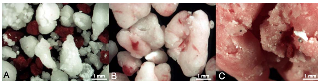
Fig. 5. Dextrin pellets (40%, w/w, water) in the equilibrium phase, plain pellets mixed with tracer pellets for different periods ( t_{\text{mix}} = 0 s (A), at t_{\text{mix}} = 60 s (B), and at t_{\text{mix}} = 200 s (C)).
